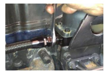
STEP 19: Utilizing the coolant bypass line riser brackets and M8 socket head cap screws in your kit; position the clamps over the bypass coolant line and fasten them to the cylinder head in the available tapped holes between cylinder numbers 2 & 3 as well as between cylinder numbers 4 & 5.
